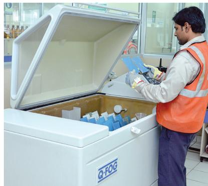
Salt Spray Corrosion Resistance Testing
