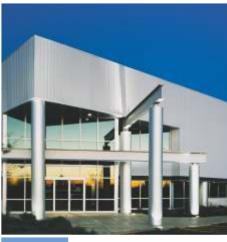
PANELRIB® 1110 is an attractive, slightly fluted wall and ceiling cladding for exterior and interior use on straight or curved surfaces. Its elegant appearance makes it suitable for many applications where a flat sheet would not normally be considered. These include ceilings, partition facings, screens, garage doors, fascias and barge boards.
